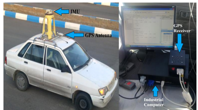
Fig. 5. Instrumented car for experiment
