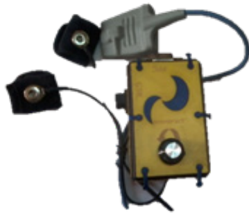
Fig. 2. The data collection unit and its sensors (PPG and GSR).
