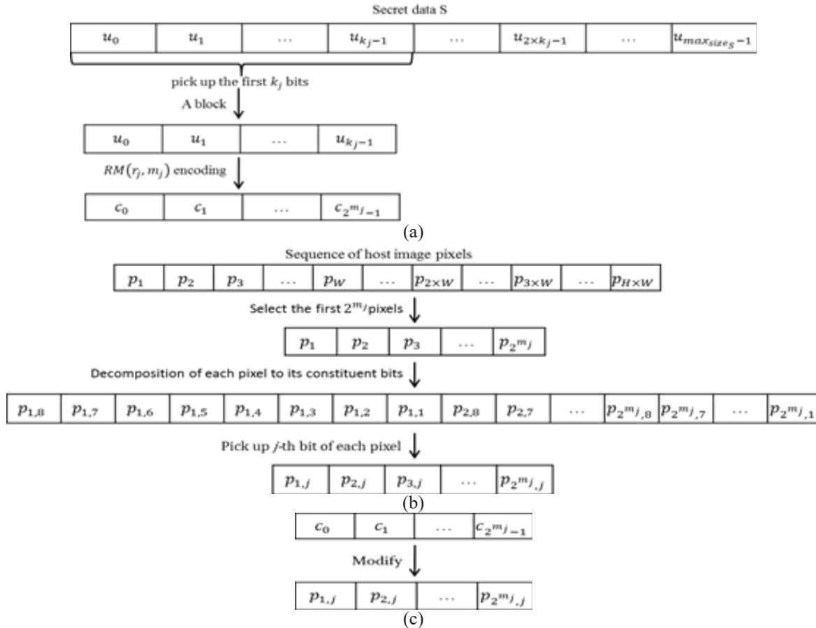
Fig. 3. Encoding process for the first information block and modifying values of the first block ( q_j=1 ) of host image: (a) generating the first information block, (b) generating the first host image block, (c) modifying.
