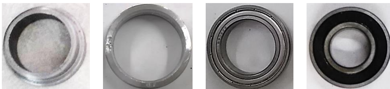
Fig. 6. Left to right: photograph of the fabricated inner ring, photograph of the fabricated outer ring, photograph of the new bearing code 6906 and photograph of the original bearing code 6205
