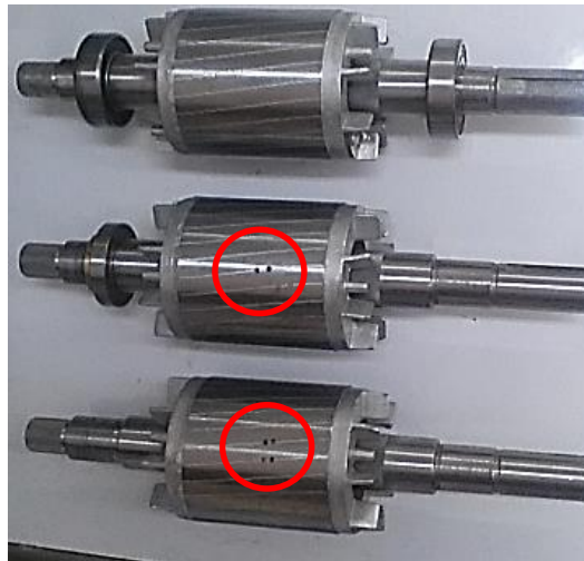
Fig. 5. Top to bottom: photograph of the healthy rotor, photograph of the rotor with one broken bar, and photograph of the rotor with two broken bars.
