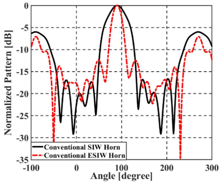
Fig. 6. The simulated H-plane radiation pattern of the conventional SIW at 27.8 GHz and ESIW antenna at 28.7 GHz.
