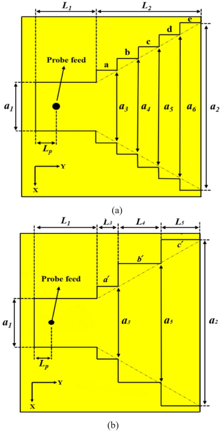
**Fig. 7. The geometry of ESIW H-plane horn using staired flaring area, a) with five sections, b) with three sections.**
