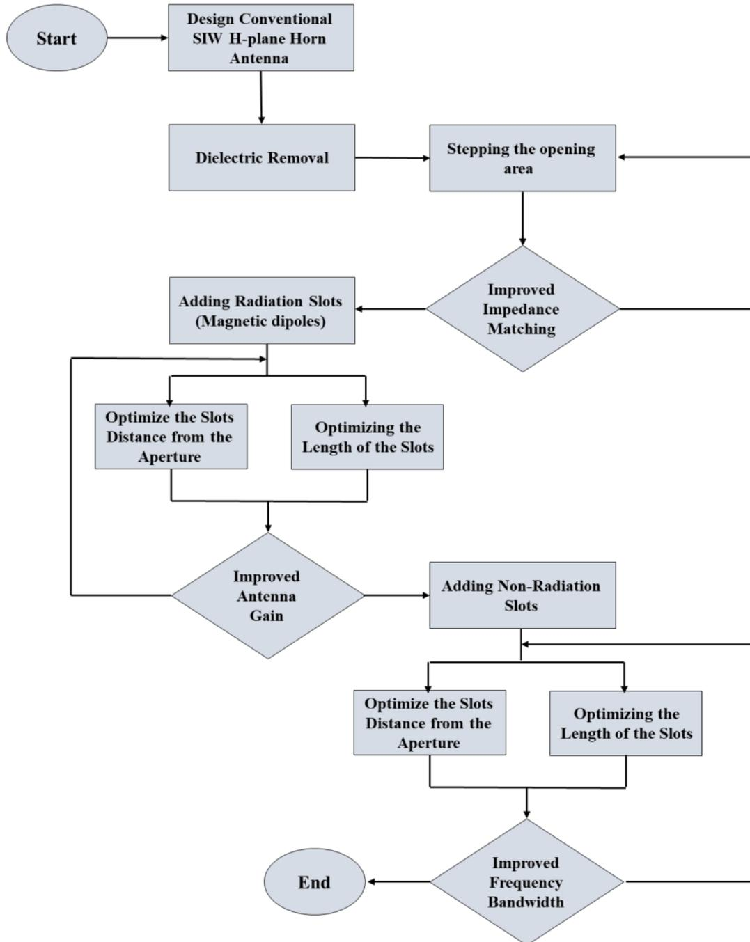
Fig. 1. The proposed procedure design of the ESIW H-plane horn antenna.
