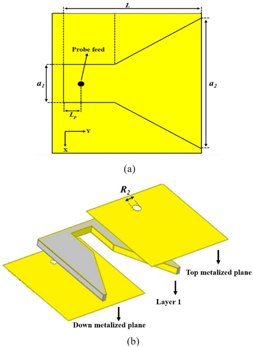
Fig. 4. The geometry of the conventional ESIW H-plane horn antenna, a) top view, b) antenna perspective.
