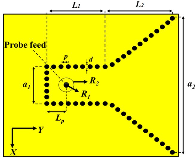
Fig. 3. The geometry of the conventional SIW H-plane horn antenna.
