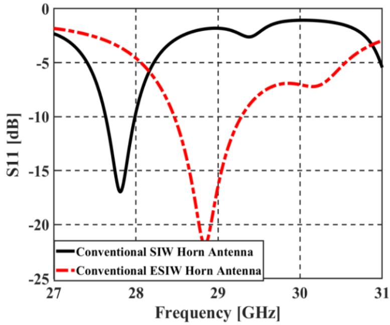
Fig. 5. The simulated  $S_{11}$  of the SIW and ESIW H-plane horn antenna versus frequency.
