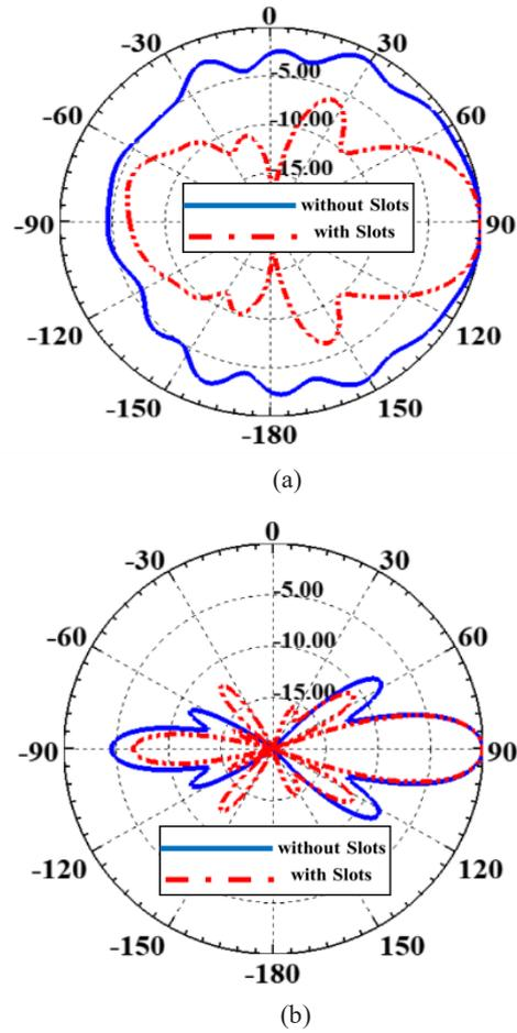
Fig. 11. The simulated radiation pattern of modified ESIW with three sections in flaring area with and without radiate at 26.5 GHz, a) E-plane, b) H-plane.
