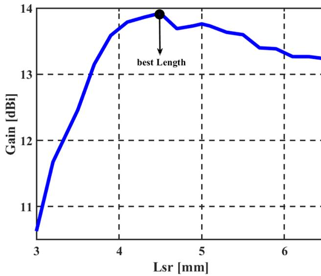
Fig. 10. The simulated antenna gain versus different lengths of the added radiating slots at 26.5 GHz.
