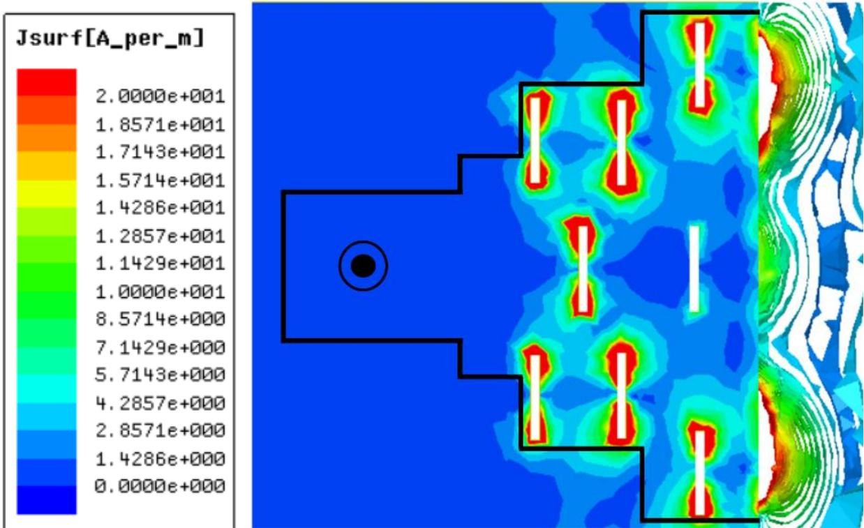
Fig. 9. The simulated distribution of the surface current and electric field from the antenna by adding radiation slots
