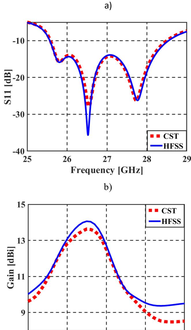
**Fig. 15.** The simulated  $S_{11}$  and gain of the ESIW with two types of slots using HFSS and CST.
