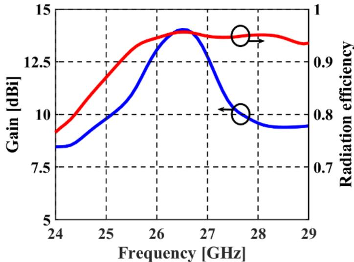
Fig. 14. The simulated gain and radiation efficiency of the proposed antenna versus frequency
