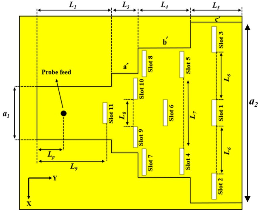
Fig. 2. The geometry of the proposed ESIW H-plane horn antenna.
