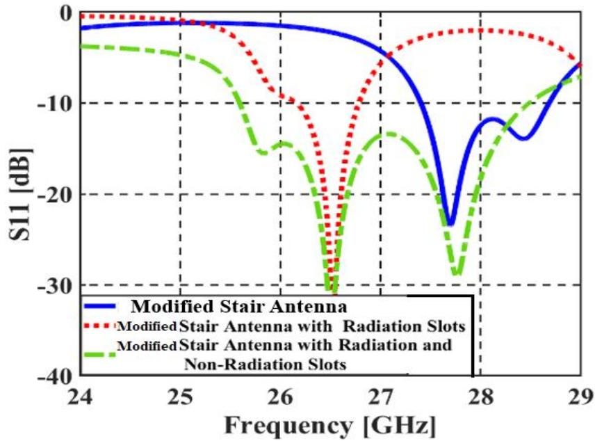
Fig. 13. The simulated  $S_{11}$  of the modified SIW horn with three sections in flaring area with and without non-radiating slots.
