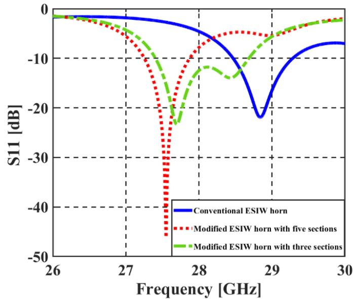
**Fig. 8. The simulated  $S_{11}$  of different horns, including conventional, modified ESIW with five and three sections in flaring area.**
