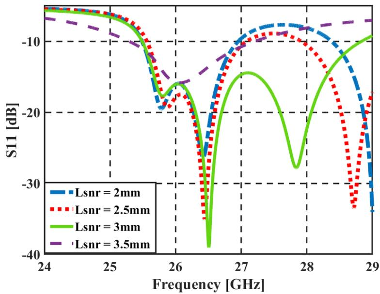
Fig. 12. The simulated S11 parameter of the antenna for different lengths of non-radiation slots.
