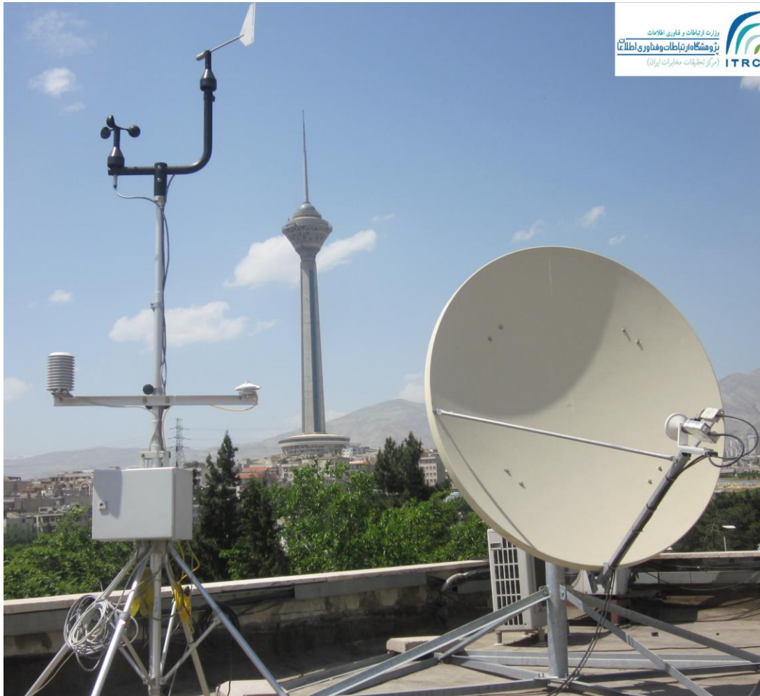
Fig. 19. The first satellite propagation study measurement setup at ITRC
