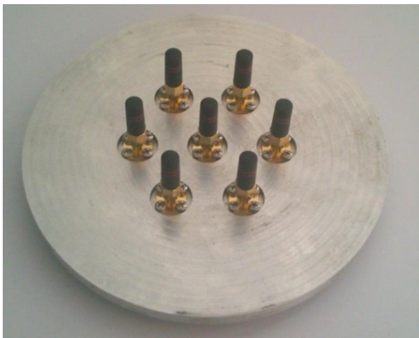
Fig. 9. The antenna set fabricated to measure the mutual coupling of ESPAR and the proposed scheme
