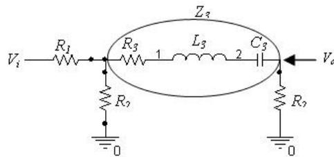
Figure 2. Electrical circuit for measuring force by tracking the output voltage changes.
