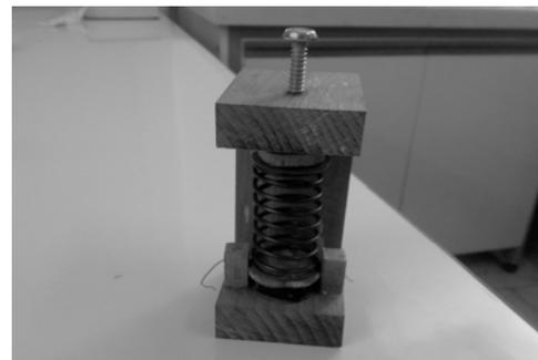
Figure 4. Designed system for sensor calibration.
