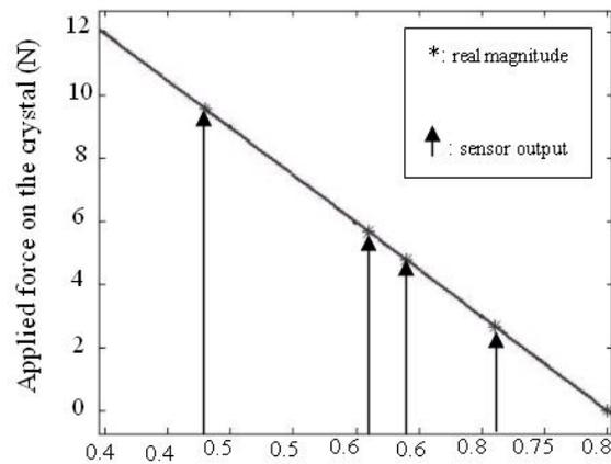
Figure 7. A comparison between calculated forces through the sensor system and the real magnitudes of the applied force.
