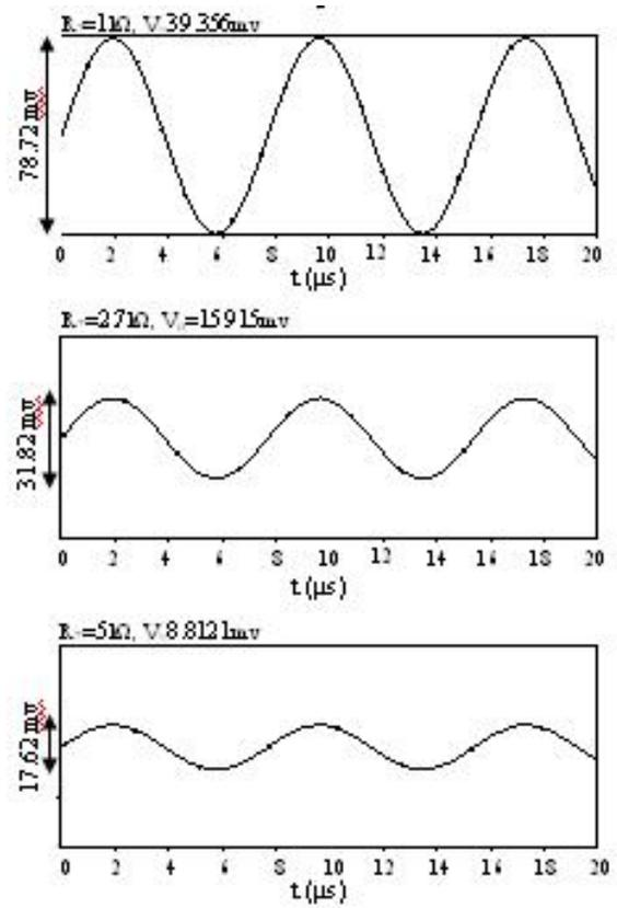
Figure 3. Changes in the output voltage as a result of impedance changing in piezoelectric.
