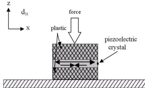
Figure 1. Applying force to piezoelectric crystal.
