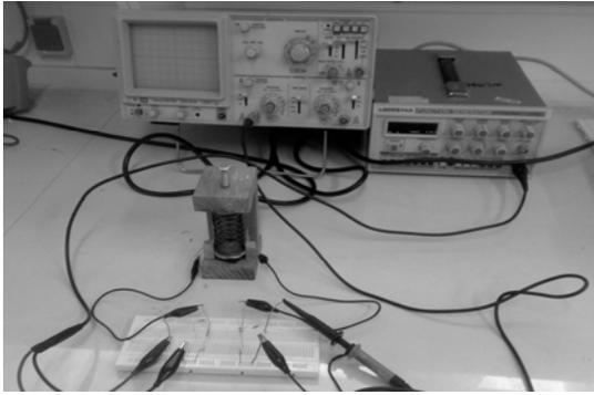
Figure 5. Applying force on the sensor and displaying the output on the oscilloscope.
