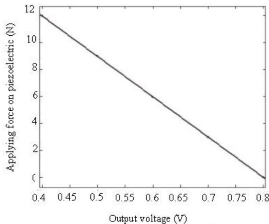
Figure 6. The graph of the magnitude of applying force on the sensor to the output voltage.
