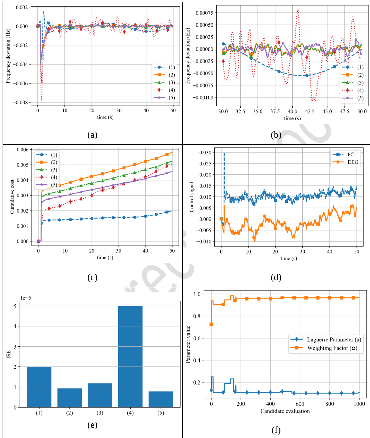
Figure 4: Performance comparison under 1% SLP: (a) frequency response, (b) zoomed frequency response, (c) cumulative cost, (d) control signals, (e) ISE, and (f) convergence of a
