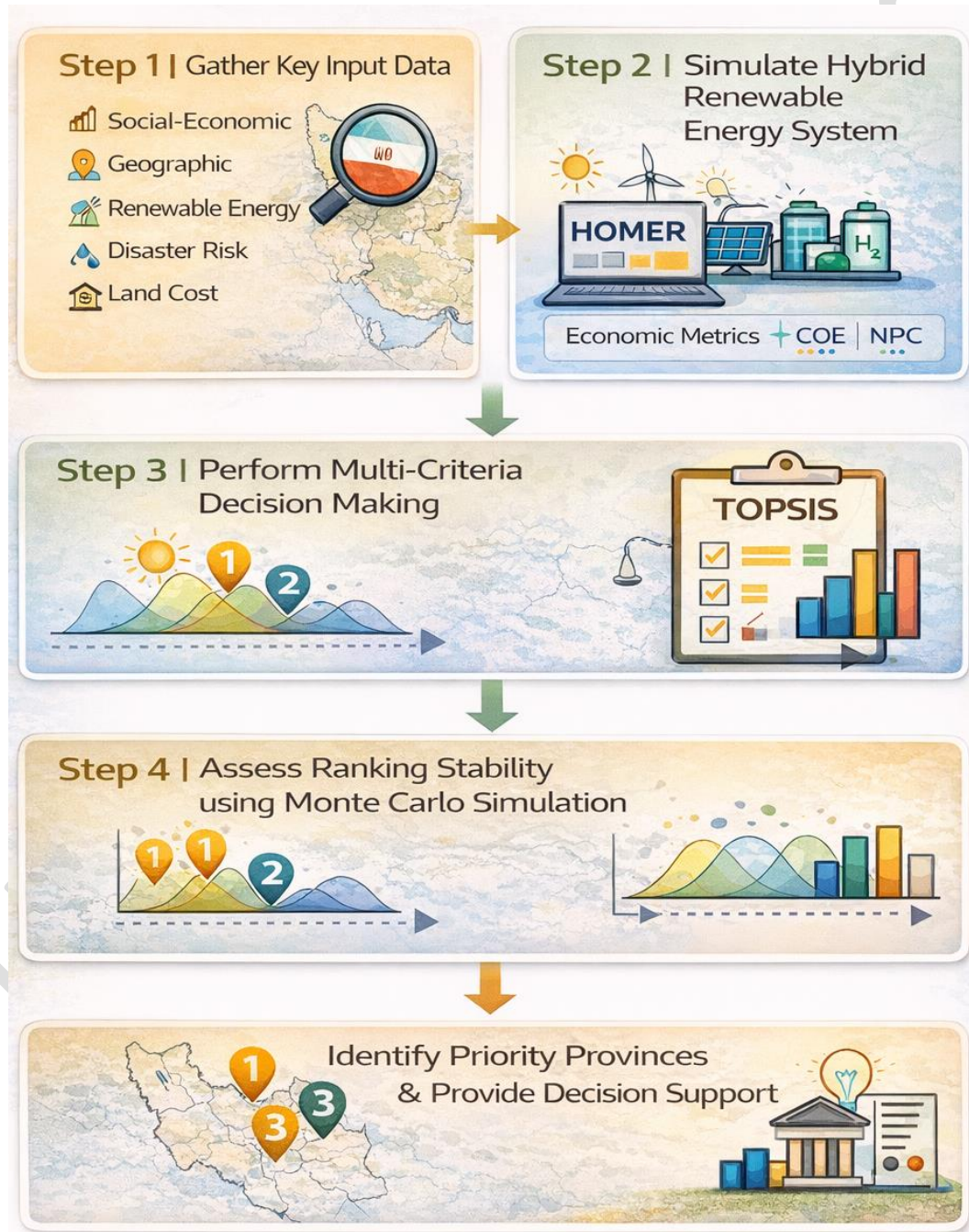
Fig. 2. Integrated framework for assessing and spatially prioritizing a solar–wind–fuel cell hybrid system based on HOMER simulation, the TOPSIS method, and Monte Carlo uncertainty analysis
