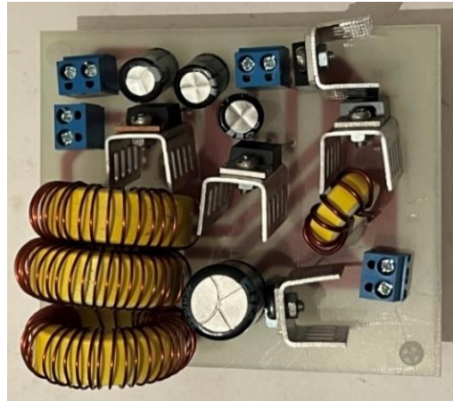
Fig. 12. Image of the proposed implemented converter
