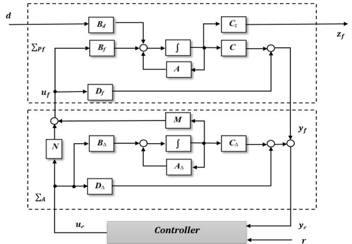
Fig. 4. Reconfigured system by means of virtual actuator.
