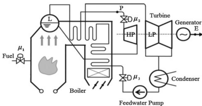
Fig. 1. Schematic of boiler-turbine unit [21]
