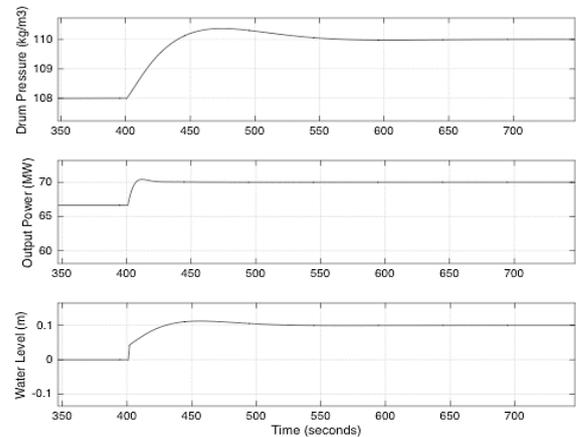
Fig. 2. Outputs of drum pressure, power and water level of the boiler-turbine unit for tracking a setpoint in closed loop form.
