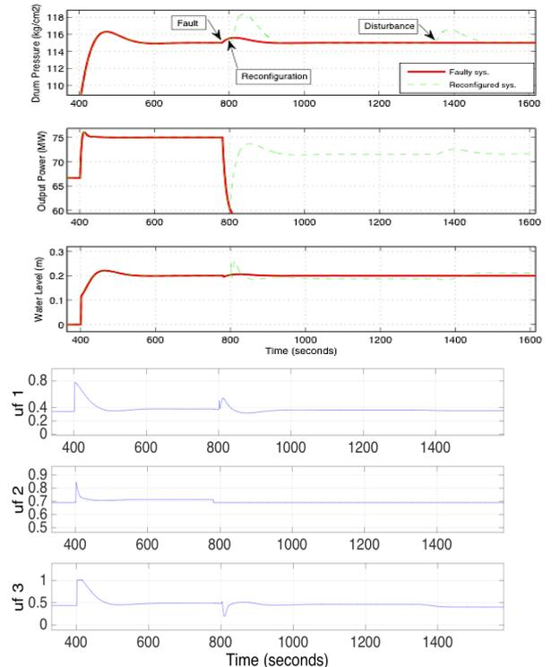
Fig. 10. Optimal performance recovery after fault  $f_2$
