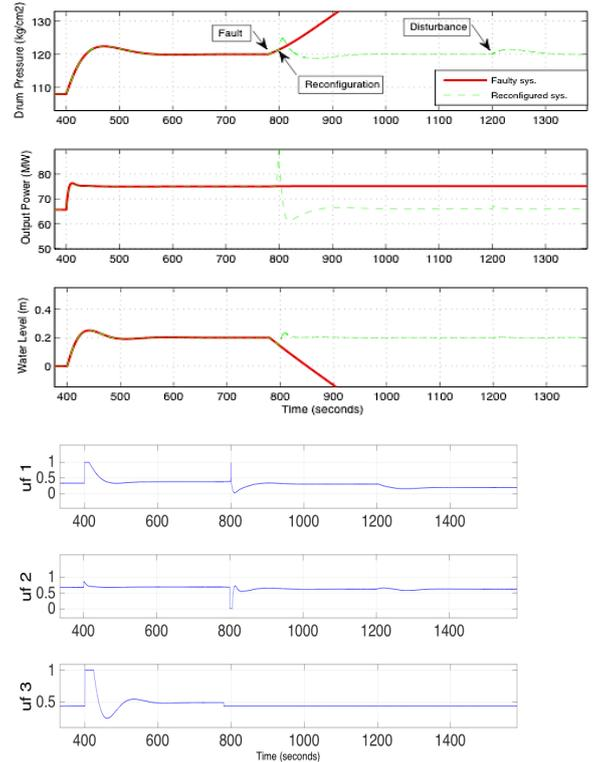
Fig. 11. Exact setpoint tracking recovery after fault  $f_3$
