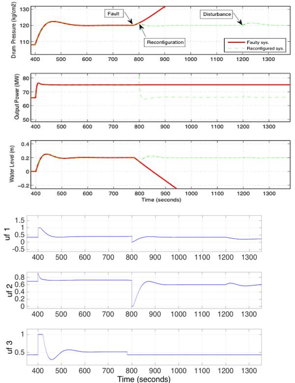
Fig. 12. Optimal performance recovery after fault  $f_3$
