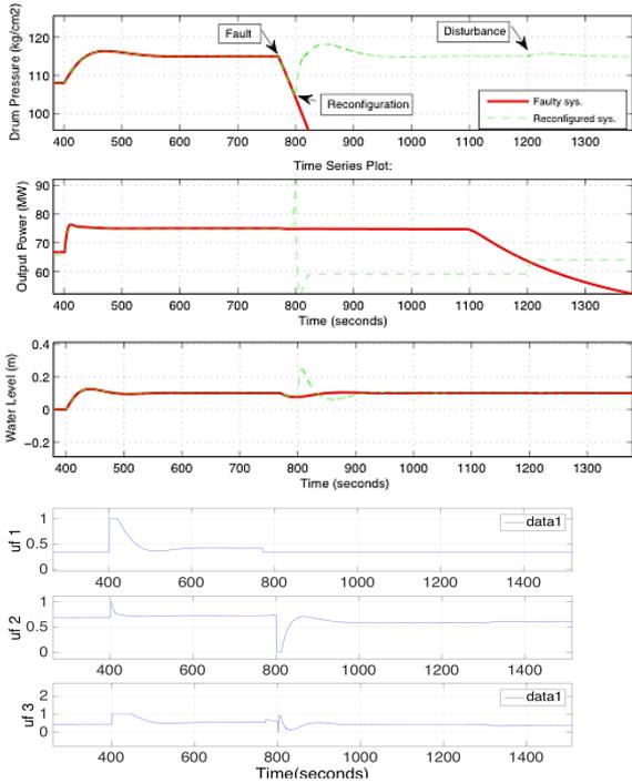
Fig. 7. Exact setpoint tracking recovery after fault  $f_1$
