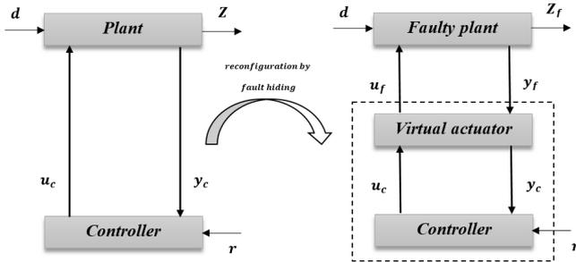
Fig. 3. Reconfiguration by fault-hiding approach
