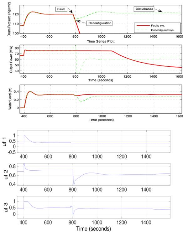
Fig. 8. Optimal performance recovery after fault  $f_1$
