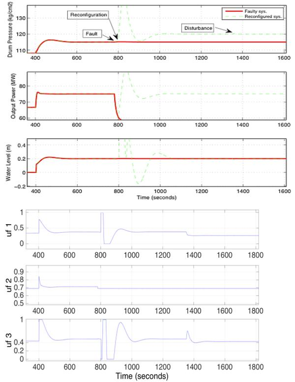
Fig. 9. Exact setpoint tracking recovery after fault  $f_2$
