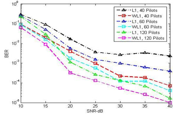
**Fig. 2. Impact of channel Side Information on BER of OFDM system,  $l_1$ -minimization**
