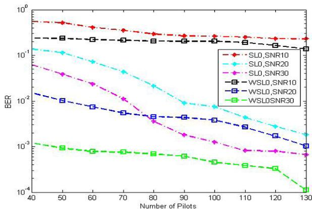
Fig. 5. Impact of Side Information on Channel Estimation, Fixed SNR, WSL0 v.s. SL0
