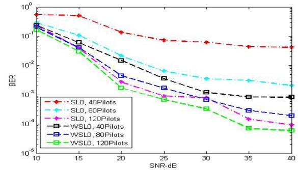
**Fig. 3. Impact of channel Side Information on BER of OFDM system, WSL0-algorithm**
