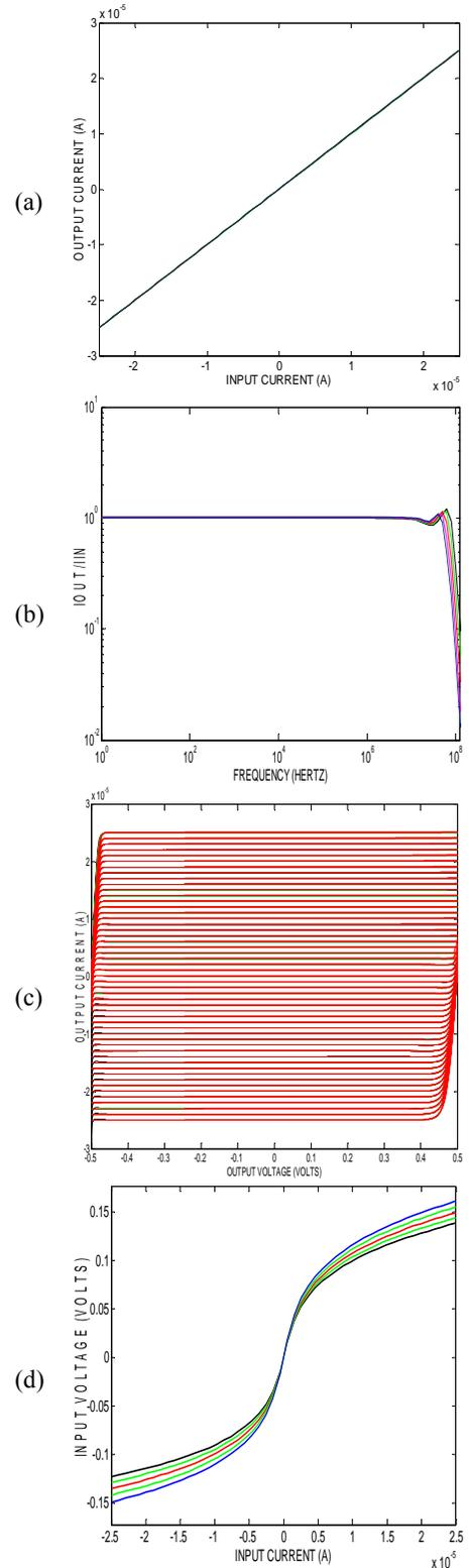
Figure 13: Temperature analysis of the proposed COS structure (a) current transfer function, (b) frequency response, (c) output current in terms of output voltage variation, and (d) input voltage in terms of input current variation.
