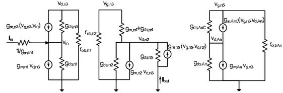
Figure 5: Half small signal equivalent circuit.
