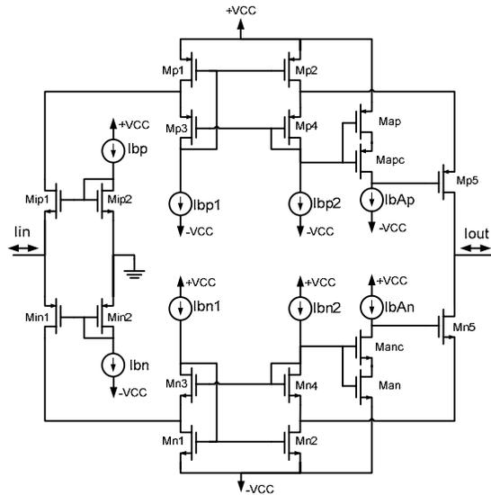
Figure 4: The transistor level schematic of a class 'AB' COS.
