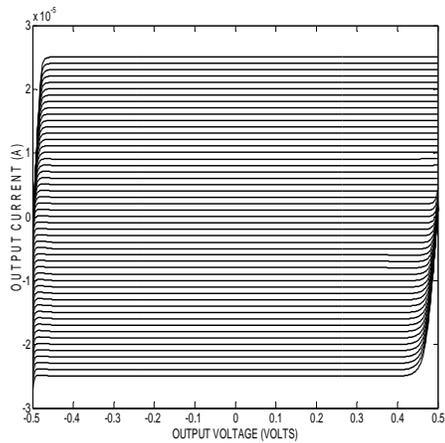
Figure 7: Output voltage of the proposed COS structure in terms of output current with input current swept from  $-25\mu\text{A}$  up to  $25\mu\text{A}$  in  $1\mu\text{A}$  steps.
