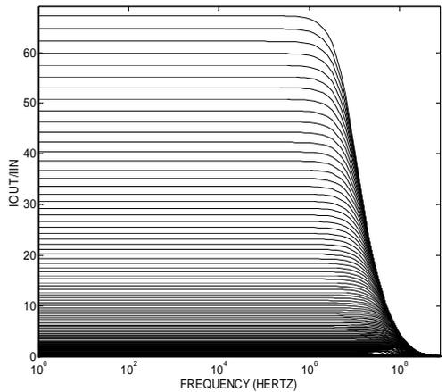
Figure 11: Frequency response of the proposed COS structure for various gains.
