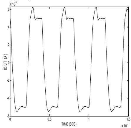
Figure 8: The transient step response of the proposed COS structure.
