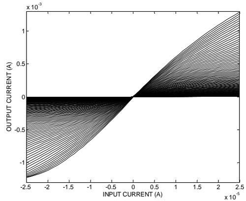
Figure 10: Current transfer function of the proposed COS structure for various gains.
