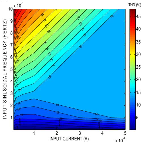
Figure 9: Total harmonic distortion of the proposed COS structure in terms of sinusoidal input current.
