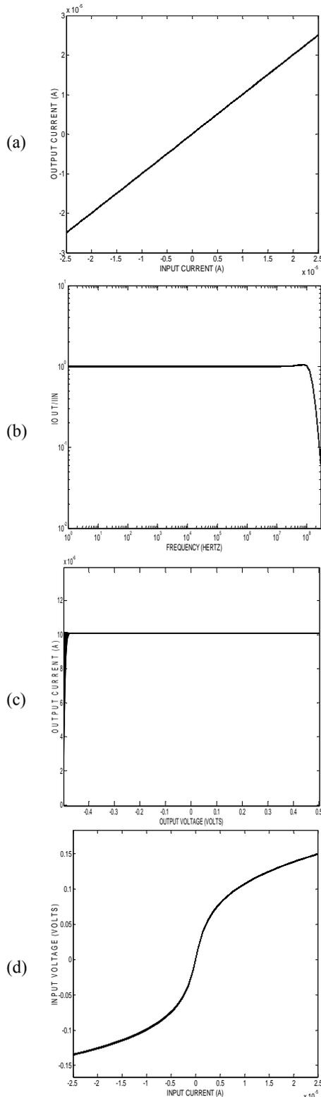
Figure 14: VDD variations analysis of the proposed COS structure (a) current transfer function, (b) frequency response, (c) output current in terms of output voltage variation, and (d) input voltage in terms of input current variation.
