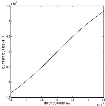
Figure 6: Current transfer function dynamic range of the proposed COS structure.
