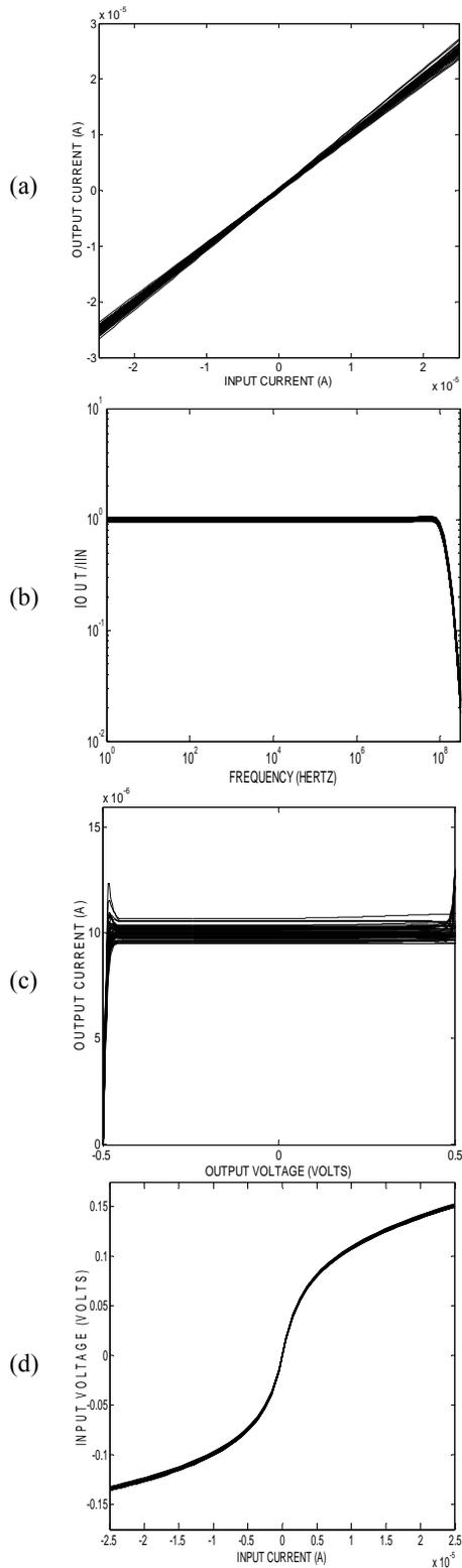
Figure 12: Monte Carlo analysis of the proposed COS structure (a) current transfer function, (b) frequency response, (c) output current in terms of output voltage variation, and (d) input voltage in terms of input current variation.
