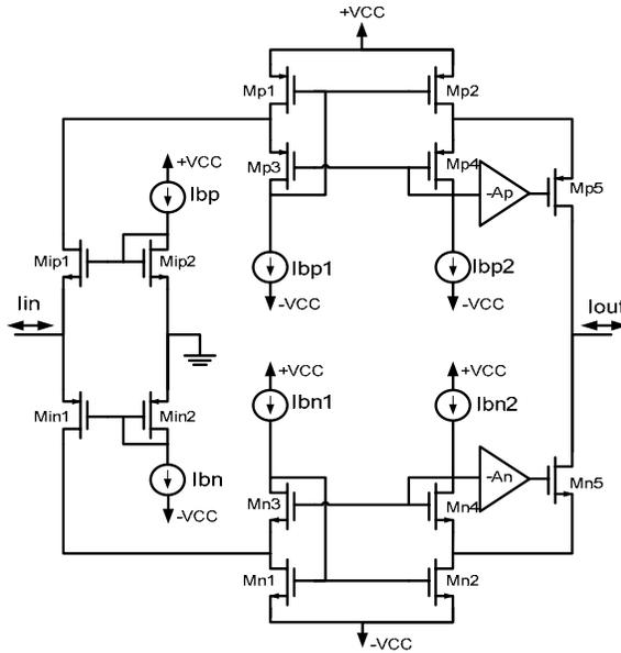
Figure 3: The conceptual schematic of a class 'AB' COS.
